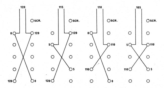
FIGURE 1 - TRANSFORMER PRIMARY CONNECTIONS.
